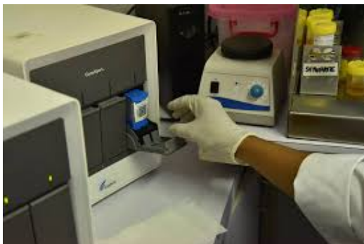
Fig. 2. A Cepheid GeneXpert device. Source: MSF (2022) [13].
